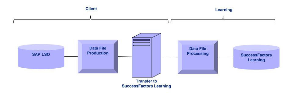
SuccessFactors Learning standard connectors are built on a producer-consumer model that requires all data input files to match a standard pre-defined format. This makes the connectors agnostic about the source of the data.
